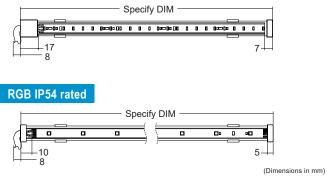
The above dimensions apply to the IP54 rated RGB Eco LD11. This is to allow extra space to connect the 4 cables to the LED board.
